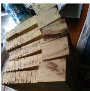
Seven new teeth ready to be inserted into the stone nut
