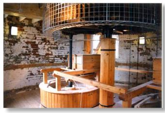
Above and around the stones is the stone furniture. The grain, in the bins above, drops down the wooden chute into the hopper, the box above the millstones. Wooden sliders in the chutes can be pushed in to stop the flow of grain.
