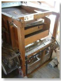
The large machine taking up much of the space on this floor is a grain cleaner. Although this one was probably made in the 1930s, Green's Mill had a similar machine during at least the latter part of its first working life. Unlike the earlier one in this mill, our grain cleaner is driven by an electric motor.
