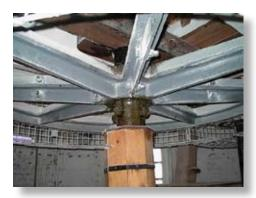
The huge gear wheel on the upright shaft is the great spur wheel. As the brakewheel (on the windshaft) and the wallower (on the upright shaft) are always in gear, whenever the sails are turning, so the great spur wheel turns as well. The spur wheel may then engage with the much smaller stone nuts, each of which is fixed to the top of the quant that will then drive a set of millstones.
