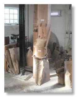
This is the floor where you will usually find the miller when the mill is at work. Here he has control over many of the parts of the mill. He can go onto the gallery to make adjustments to the sails and to get to the brake rope to stop and start the mill. As we have seen he can adjust the flow of grain into the stones by adjusting the rope supporting the the shoe. You can see it coming down from the stones above, next to the meal chute.
