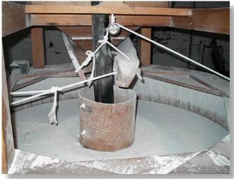
The arrangement of damsel and shoe is very elegant for it allows both manual and automatic control of the flow of grain. A windmill never runs at a constant speed for the wind itself is inconstant. As the mill speeds up in the gusts, the quant turns faster and more grain is joggled off the end of the shoe. Likewise, as the mill slows, the flow of grain slows and even stops completely if the mill comes to rest. Thus the flow of grain is matched to the speed of the mill.
